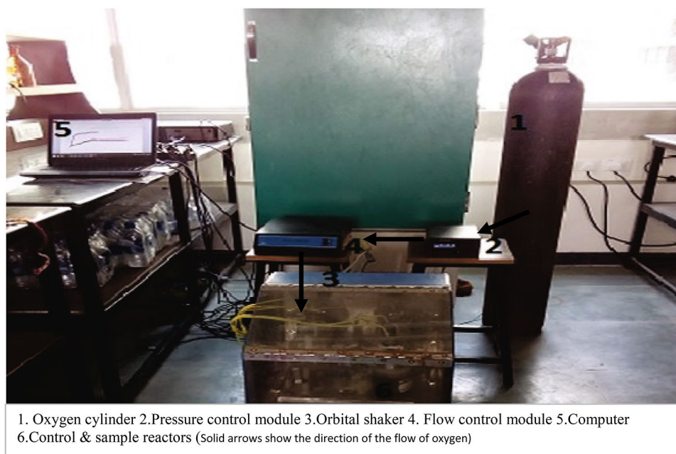
Fig. 1 Head space respirometer setup
